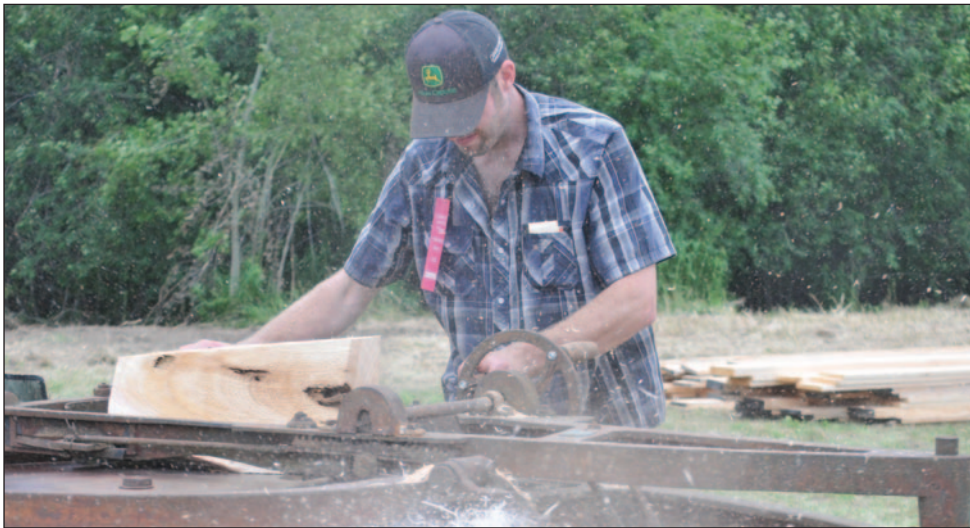
In the photo above is Nathan Baker from Roslin, operating a round shingle mill. This is the first step in a process to make shingles in the late 1800's. Nathan works in the trades today and "enjoys simpler times" operating heritage equipment like this. Nathan is a member of KAP, and enjoyed participating in the show.
