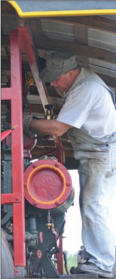
In the photo above is Nathan Baker from Roslin, operating a round shingle mill. This is the first step in a process to make shingles in the late 1800's. Nathan works in the trades today and "enjoys simpler times" operating heritage equipment like this. Nathan is a member of KAP, and enjoyed participating in the show.
