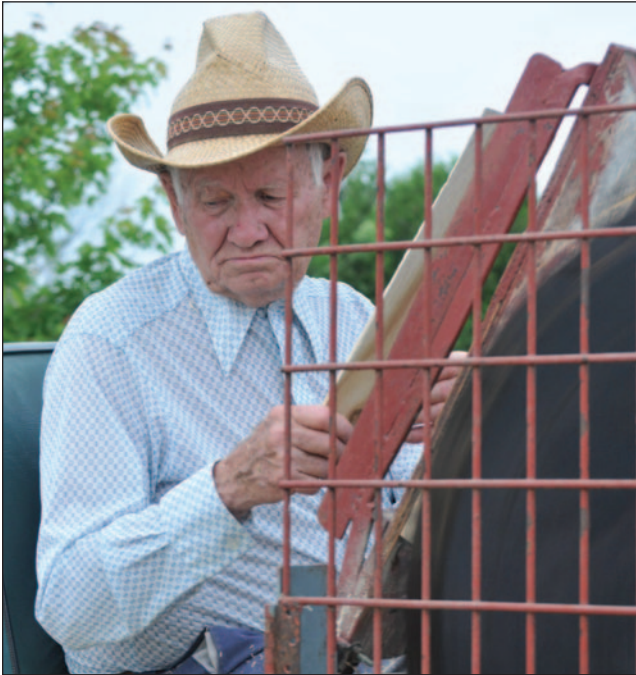
This is Eric Ward making shingles on a Shingle Mill owned by the Durham Heritage Gas & Steam Society at the Kawartha Antique Power 45th Annual Heritage Show. These shingles are being made from cedar that has been in dry storage for three years. The shingles are a club fundraiser as they are sold to be used on garden sheds.
