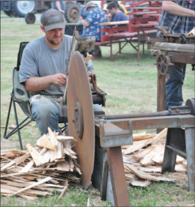
In the photo above is Josh Struik operating the edger which is the second part of a shingle mill operation, which does the finishing. Beside is the "bundler" which is like a wooden box with a lever on it that puts the shingles into a uniform bundle. All of this heritage equipment is from the 1800's and is currently owned by Nathan Baker.
