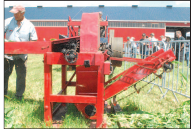
Pictured above is a Corn Chopper owned by the Lewis Family. The corn chopper was used to make corn into livestock feed. This machine was made in the 1920's.
