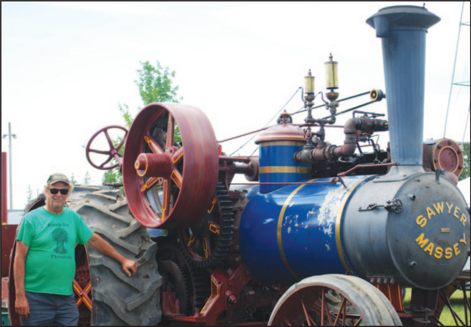
Pictured above, Frank Hume from Milton stands beside his 68 horsepower Sawyer Massey Steam Traction Engine. This Steam Engine was made in 1913 and it would have cost between $3,000 to $4,000. Frank's farm is the site for the 61st Steam Era Show that takes place on Labour Day Weekend hosted by the Ontario Steam & Antique Preservers Association. Steam Era features steam powered tractors, engines and farm implements and is considered the biggest exhibition of antique steam powered equipment in Ontario.
