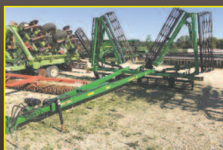
JD 200 (E83473) 2010, 45', SOIL CONDITIONER, 14"DIA. HYDRAULIC LIFT, SINGLE ROUND BAR BASKET, 5-SECTION DOUBLE FOLD, TELESCOPIC TONGUE, SINGLE TRANSPORT WHEELS $19,900.00
