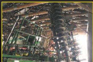
JD 726 (E85704) 2003, 33.9', MULCH FINISHER, 7" SPACING, C-SHANK, 7.5" SWEEPS, KNOCK-ON SWEEPS, 20% REMAINING, HYD GANG DEPTH ADJ, ROCK-FLEX GANG, 19"BLADE DIA $30,000.00
